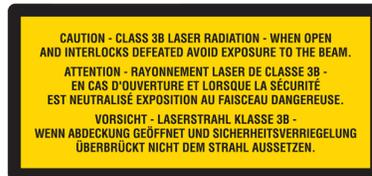
Laser beam class 3B when covers are removed
