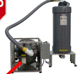
1) Confirm the voltage is between 220-240 Volts AC (record voltage below)\*
